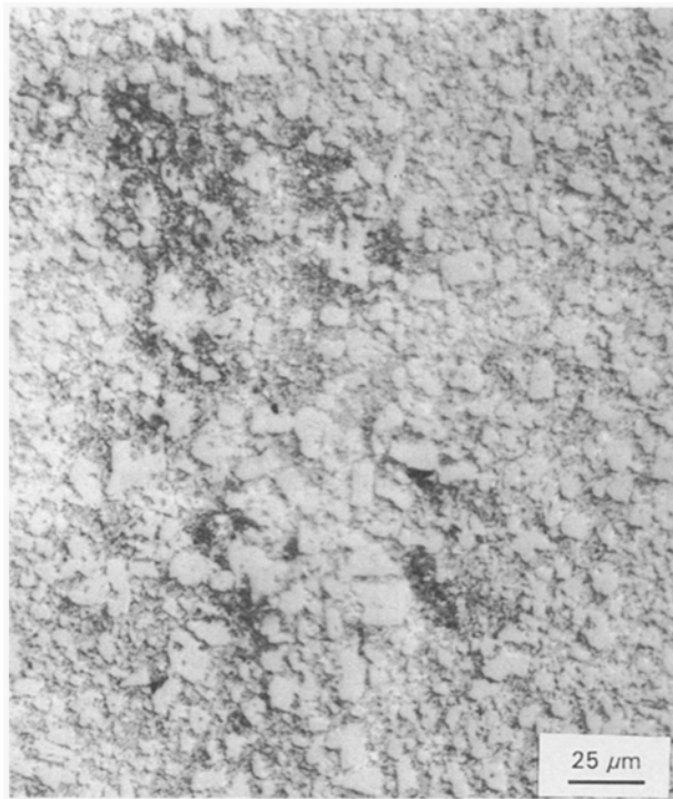
Figure 7 Optical micrographs of the Al-40Si composite (Sumitomo).
